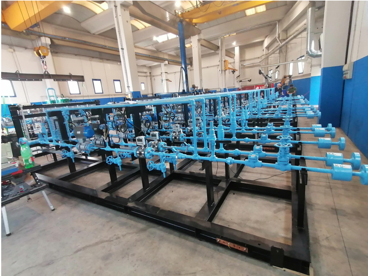
Finger Manifold SKID
