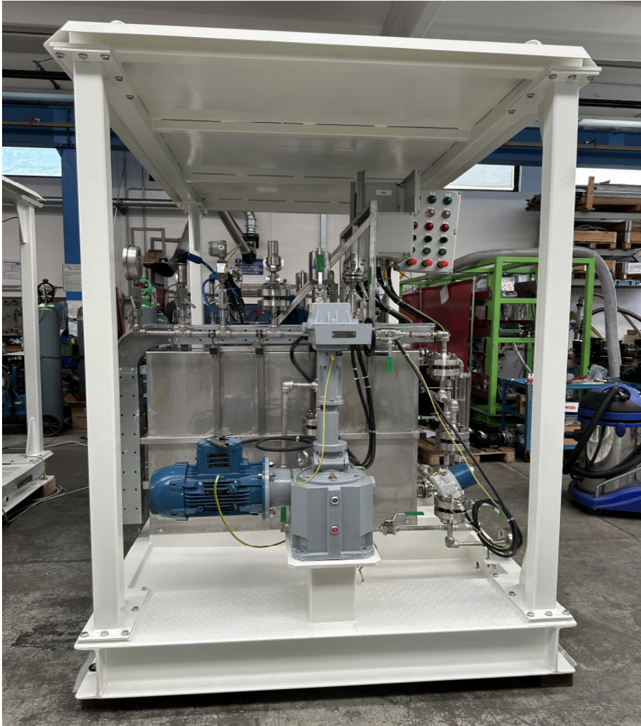
Chemical dosing skid
